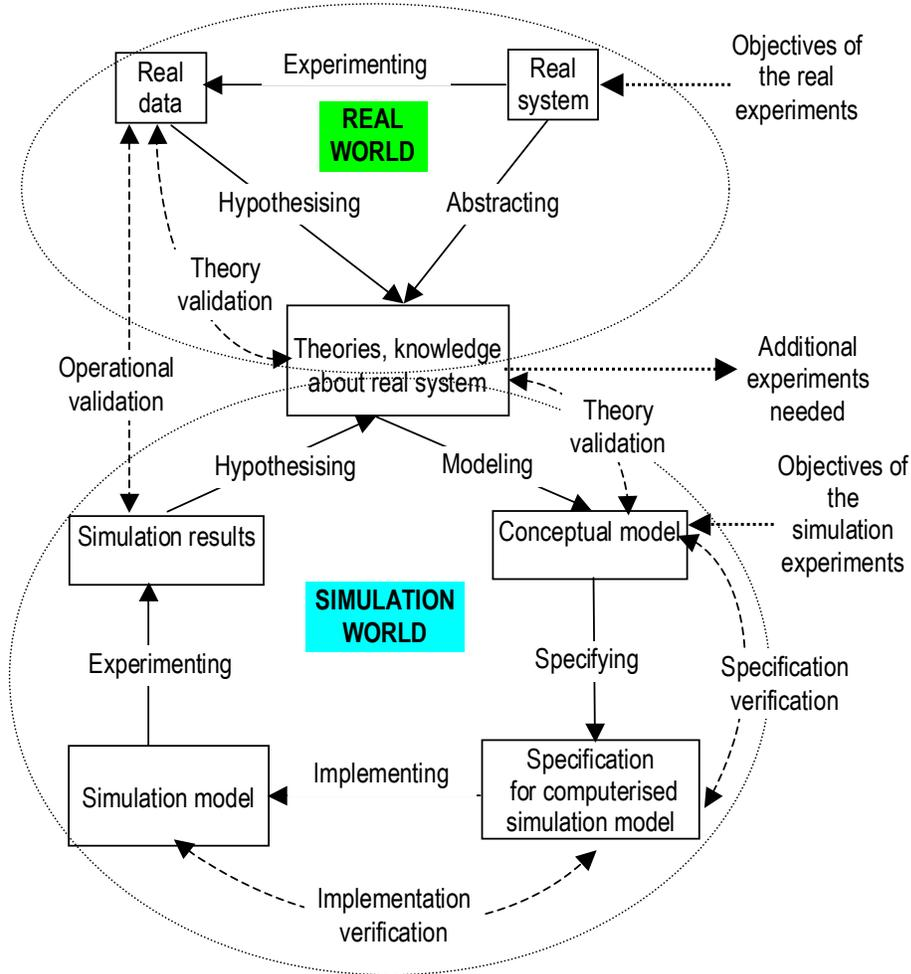
FIGURE 1 – SIMULATION MODEL DEVELOPMENT PROCESS
