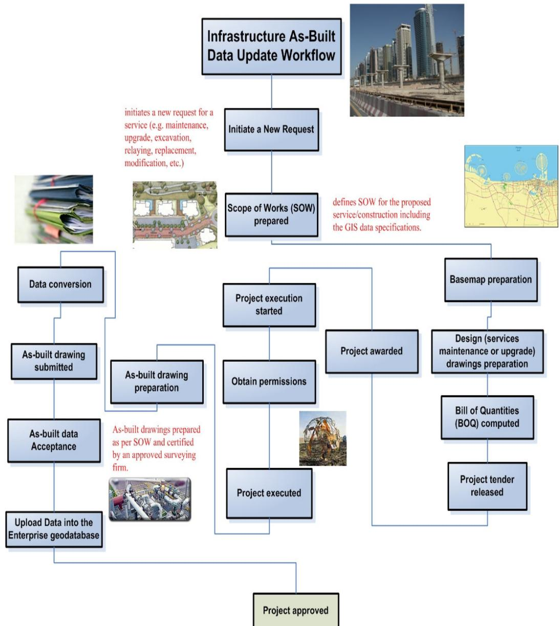
FIGURE 3. CITY INFRASTRUCTURES MONITORING AS-BUILT DATA UPDATE WORKFLOW
