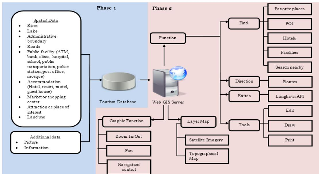
FIGURE 1 - CONCEPTUAL DESIGN OF WEB GIS LANGKAWI
