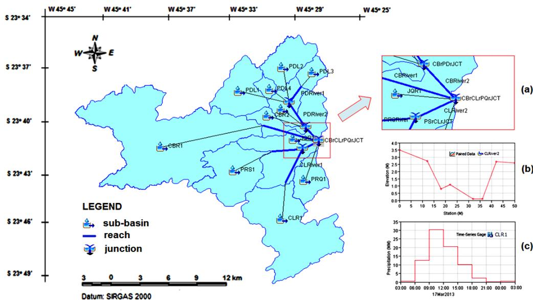
FIGURE 3 - (A) HYDROLOGICAL ELEMENTS OF A BASIN MODEL. (B) PAIRED-DATA: THE CROSS-SECTION OF THE CLARO RIVER REACH (CLRIVER2). (C) TIME-SERIES DATA: PRECIPITATION HYDROGRAPH OF THE CLARO RIVER SUB-BASIN (CLR1).
