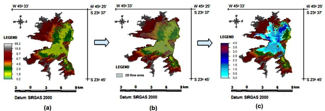
FIGURE 4 - HEC-RAS 2D: (A) TERRAIN MODEL. (B) 2D FLOW AREA. (C) FLOOD SIMULATION.
