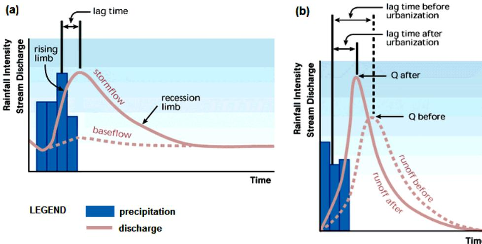
FIGURE 2 - (A) COMPONENTS OF THE STORM HYDROGRAPH. (B) URBANISATION EFFECTS ON THE STORM HYDROGRAPH. SOURCE: ADAPTED FROM USEPA (2017)
