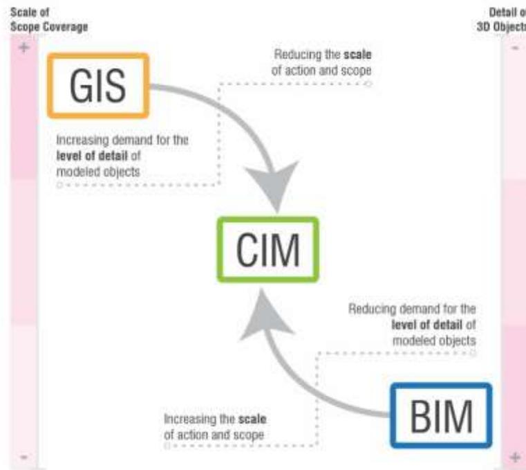
FIGURE 2 – THE RELATIONSHIP BETWEEN GIS, BIM, AND CIM FROM THEIR COMPREHENSIVENESS SCALE AND THE DETAIL LEVELS OF THEIR THREE-DIMENSIONAL OBJECTS
