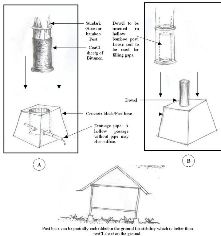
FIGURE 6. PROPOSED CONCRETE BLOCKS FOR PROTECTING BAMBOO POSTS
