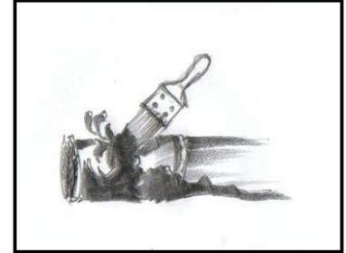
FIGURE 5C: SOAKING IT IN BITUMEN FOR 24 HOURS
