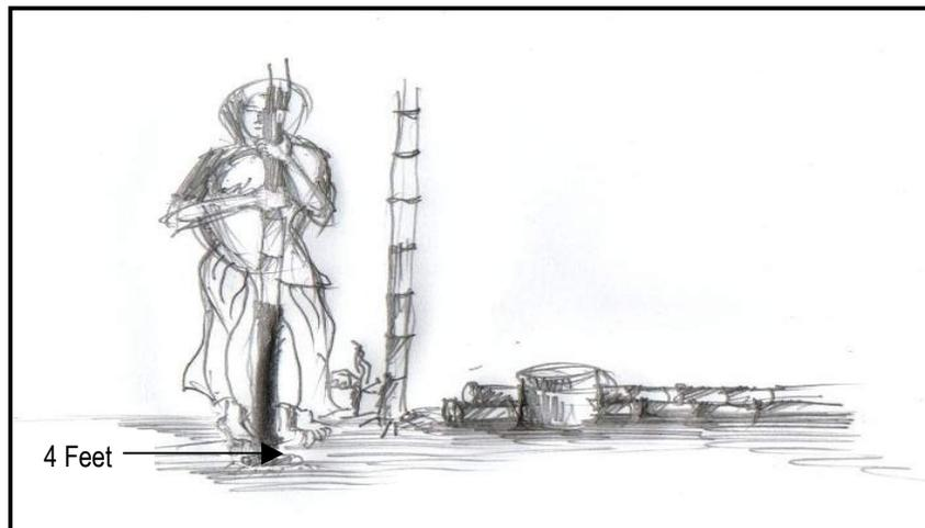
FIGURE 5. PROPOSED TREATMENT OF BAMBOO POSTS TO BE EMBEDDED INTO THE GROUND
