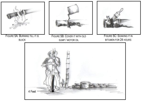
FIGURE 5. PROPOSED TREATMENT OF BAMBOO POSTS TO BE EMBEDDED INTO THE GROUND Adapted from Ahmed, 1994
