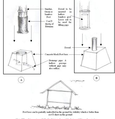
$\underline{Note:}$  Where bitumen is available detail A is to be used for better stability and protection.
