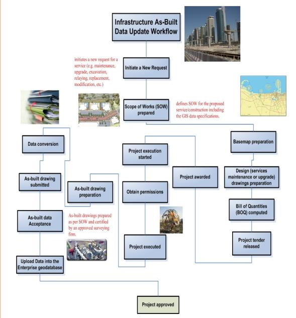
FIGURE 3. CITY INFRASTRUCTURES MONITORING AS-BUILT DATA UPDATE WORKFLOW
