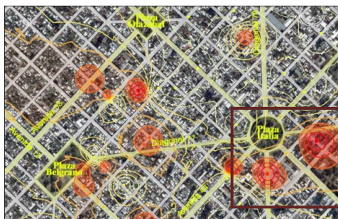
FIGURE 11 - FLOOD AREAS AT CENTRAL URBAN AREA
