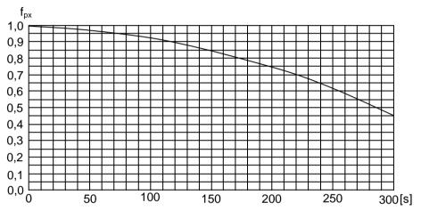
$\label{eq:Figure 2-The coefficient for the proportion of pedestrian crossings (Source: Transit Capacity and Quality of Service Manual – 2nd Edition, TRB 2003)$
