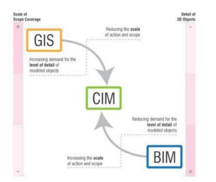
FIGURE 2 – THE RELATIONSHIP BETWEEN GIS, BIM, AND CIM FROM THEIR COMPREHENSIVENESS SCALE AND THE DETAIL LEVELS OF THEIR THREE-DIMENSIONAL OBJECTS
