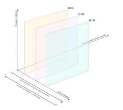
FIGURE 5 – ANALYTICAL FRAMEWORK OF THE CIM ECOSYSTEM CONSIDERING THE TECHNOLOGICAL FIELDS DELIMITED FOR GIS, CIM, AND BIM.
